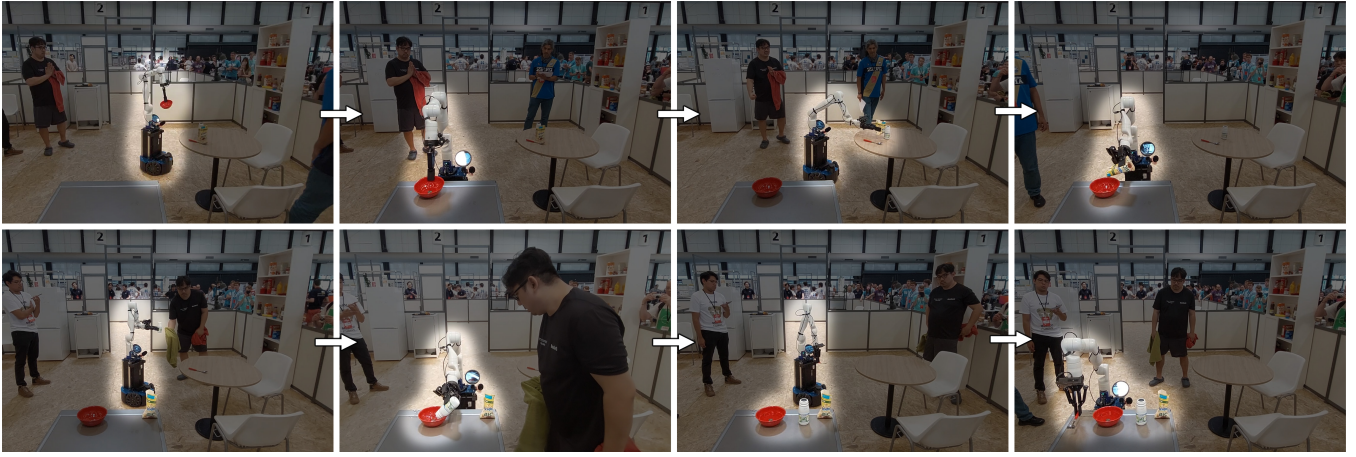
Fig. 4: Making Breakfast Task: During the RoboCup@Home competition, a single-arm mobile manipulator carries out a multi-step breakfast setup involving (i) bringing a bowl and placing it on the table, (ii) fetching cereal and setting it down, (iii) retrieving milk and pouring it into the bowl, and (iv) bringing a spoon and placing it alongside. Eight time-lapse frames showcase D-RDMM’s ability to orchestrate long-horizon navigation, manipulation, and interaction in a realistic, human-populated environment.
